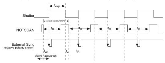
Figure 45. Overlapped Mode where  $t_{wl} + t_{exp} + t_c > t_R$
